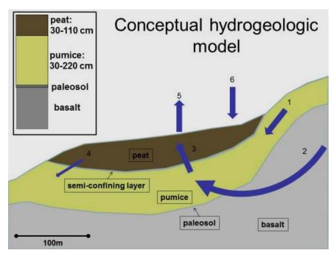
**Figure 5**. Conceptual hydrogeologic model cross section of the three study fens. Water balance elements are depicted as blue arrows: (1) shallow groundwater flow from local pumice deposits; (2) deeper groundwater flow through the basalt; (3) groundwater discharge from pumice to peat through leaky confining layer; (4) groundwater outflow from the fen to the pumice; (5) evapotranspiration; (6) direct precipitation.
