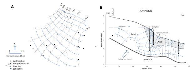
Figure 6. Flow nets generated to indicate flow of water through Johnson Fen based on water levels measured May 18, 2010. (A) plan view and (B) cross sectional view showing soils and geologic strata. Groundwater flow direction is indicated by flow lines (blue lines), and lines of equal hydraulic head (equipotential lines) are shown with dashed lines.
